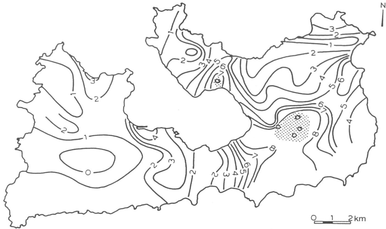
Fig. 10.4 Thermal gradient map of Milos island, Greece. The main geothermal areas (shaded zones) are characterized by large values of thermal gradient ( >8^{\circ}\text{C}/10\text{ m} ). Open circles show locations of boreholes with large steam production. (After Fytikas, 1977.)
