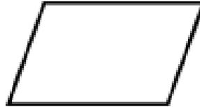
a parallelogram called input/output
